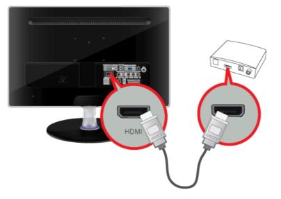
Connect the HDMI OUT port of the AV device (Blu-Ray/DVD/Cable/Satellite box) to the [HDMI IN] terminal of the monitor using the HDMI cable.
